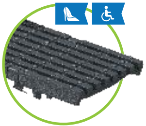
6. Ductile iron elongated bar grating MW 1.14" x 0.24" (29x6 mm) cl. C narrow MW for NW 100
