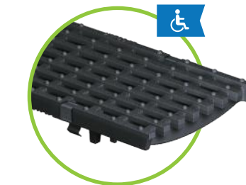
7. Ductile iron elongated bar grating MW 1.14" x 0.51" (29x13 mm) cl. C or cl. D for NW 100 to 200
