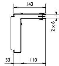
Revisionsschacht 2S / revision shaft 2S, Heelproof, SW 2x6mm, SH 110, C250
