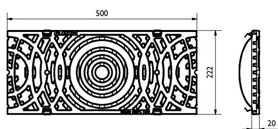
Gußrost / Ductile iron grating: SW2x14/95, F900
