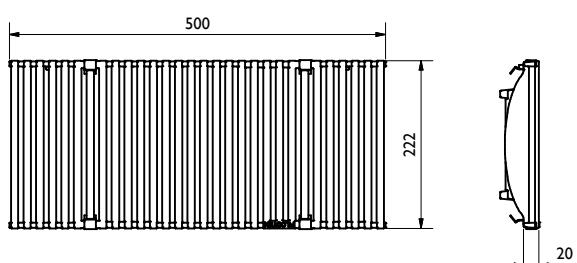
Guß-Stegrost / Ductile iron slotted grating: SW14/150, E600
