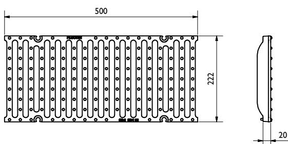
Gußrost / Ductile iron grating: MW22/13, E600
