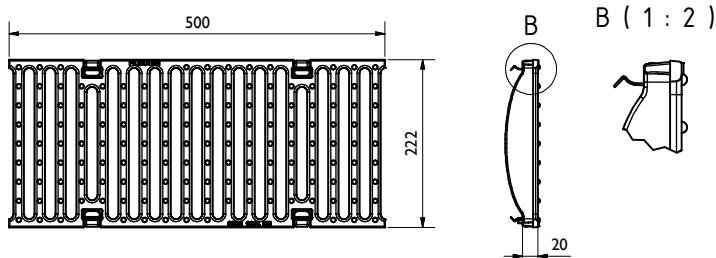
Guß-Stegrost / Ductile iron slotted grating: SW14/200, D400
