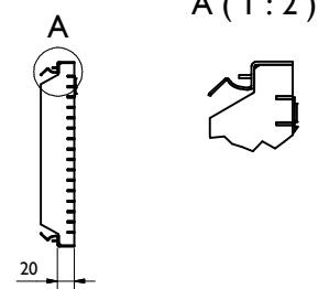
Gitterrost / Mesh grating: MW25/10, D400
