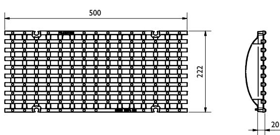
Gußrost / Ductile iron grating: MW29/13, D400
