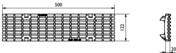
Gußrost / Ductile iron grating: MW 29/13, D400
