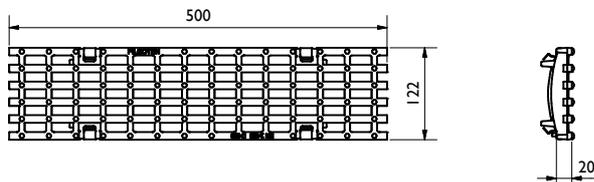
Guß-Stegrost / Ductile iron slotted grating: SW 14/100, E600
