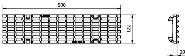
Gussrost / Ductile iron grating: MW29/6, C250
