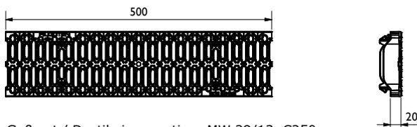
Gußrost / Ductile iron grating: MW 29/13, C250
