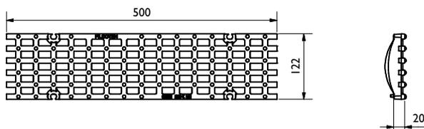
Guß-Stegrost / Ductile iron slotted grating: SW 14/100, D400
