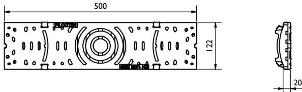
Gußrost / Ductile iron grating: MW 22/13, E600
