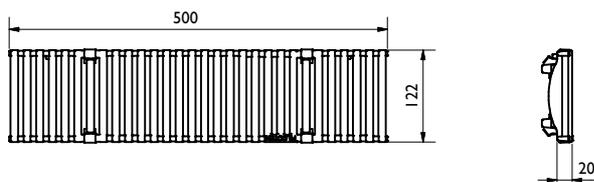
Guß-Designrost / Ductile iron design grating: VIA, D400
